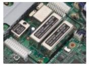
these IF filters can be installed inside the transceiver.
